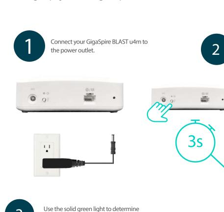
Once the light begins flashing red, you can pair your GigaSpire BLAST u4m (extender) with the GigaSpire BLAST u6x (router).
